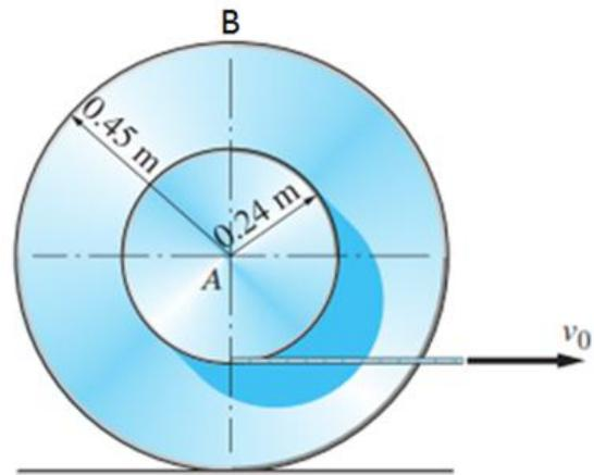
$$\begin{aligned} \vec{V}(I) &= 0 = \vec{V}(A) + \vec{\omega} \wedge \vec{CI} = 0 \\ &= v_0 \vec{y} + \vec{\omega} \wedge (R - r) \vec{x} \\ &= (v_0 - \omega(R - r)) \vec{y} = 0 \\ \rightarrow \omega &= \frac{v_0}{R - r} \end{aligned}$$
